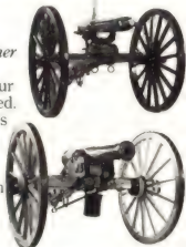
The Weapons The war spurred such innovations as the model 1863 Gatling gun (top), submarines and reconnaissance balloons. The barrel of this smoothbore 6-pounder (bottom) was rifled for extra accuracy and range.
